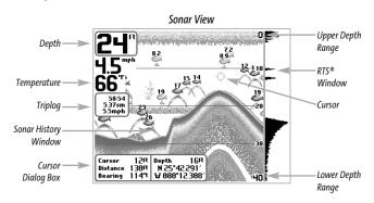
**NOTE:** If the Depth number is flashing, it means that the unit is having trouble locating the bottom. This usually happens if the water is too deep, the transducer is out of the water, the boat is moving too fast, or for any other reason that the unit can't accurately receive continuous data.
